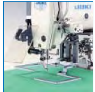
LK-1920SA (Pneumatic separately driven feeding frame)
